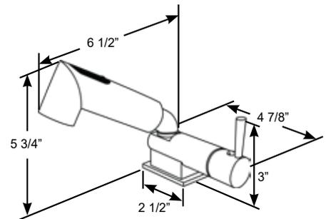
**Minimalistic** single lever design combination faucet and shower mixer. Press the button on back of handle to switch between aerated water flow or shower spray. Ceramic valve. Features inward opening valve handle to prevent accidental opening in rough conditions while underway.
