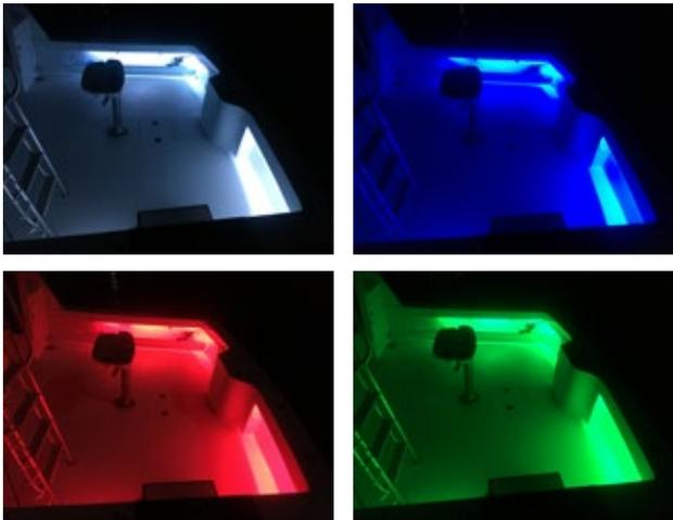
Scan-Strip 4-Color RGBW LED builds on the popularity of our original single color Scan-Strip LED. Simple 2-wire connections with any on/off switch is all that is required to cycle from White to Blue to Red to Green. Switch off for more than 4 seconds resets the color to white.
