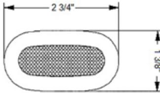
**LED Surface Mount Courtesy Light.** ABS housing with white or stainless steel snap on trim. 5 x 0.4 Watt white LEDs (4,500K) or 5 TOP blue LED's. LED beam angle is 120°. White is 15 lumens and blue is 2.8 lumens. 12 V, IP65. Dimensions 2-7/8" L x 1-1/2" W x 7/16" D.
