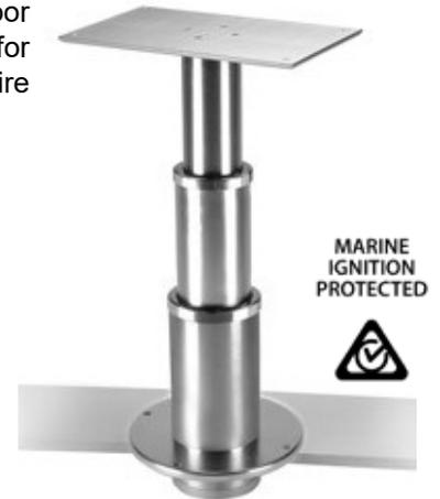
**Two-stage 6" Electric Pedestal with sliding upper plate to adjust table distance from seating.** Built in polished, brightened and anodized light alloy Sliding upper plate with 7.8" stroke to adjust the table distance from seating The generous size of the tubes and bases make it ideal for tables of large dimensions. The two stages telescope enables to get a reduced minimal height, often necessary to transform a table in bed. Push 220 lbs.
