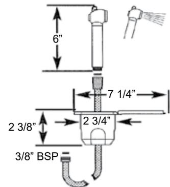
**Euro Style ABS sprayer**, chrome or white. Convenient on/off trigger locks in the "on" position for continuous water flow. Mounting hardware included.
