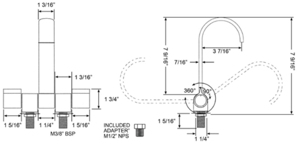
**NEW Folding Square Ceramic Mixer** Built on the platform from the Folding Ceramic Family, we have added the square spout from the Geometric Family. A ceramic valve cartridge, for drip free service, is mated with a chrome ABS knob for precision performance.
