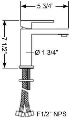
**Farley Single Lever Basin Mixer.** Ceramic valve. Included pop-up drain fits 1-7/8" drain hole, has 1-1/4" threaded outlet.
