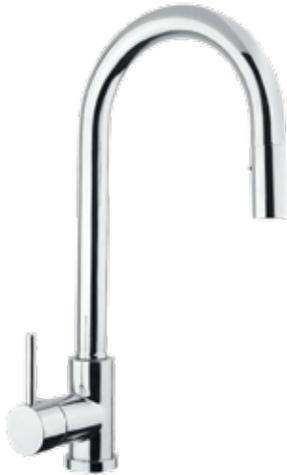
**Nordic Family, Chrome Galley Faucet with Ejectable Handle.** Tall J spout provides 9 5/8" of clearance from spout tip to the counter top. Single lever water control is mated to a ceramic valve cartridge for trouble free operation.
