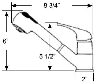
Basin mixer with pull-out handle. Push button compact galley or spray pattern adjustment located on handle. 5' chrome flex hose. This faucet does **NOT** swivel. Ceramic valve.
