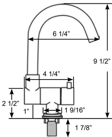
**J-Spout Stainless Steel Folding**, Swivel Spout, **COLD WATER** tap. Ceramic valve.
