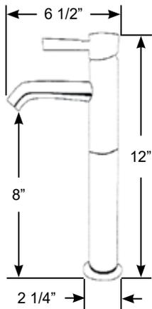
**Nordic Family** Raised Deck Mount Mixer for vessel sinks. Ceramic valve.
