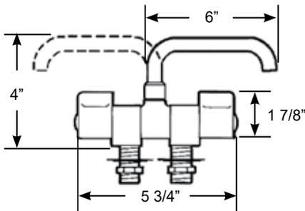
**Water Connection:** 3/8" BSP-M threaded shafts, 1/2" NPS-M adapters included
