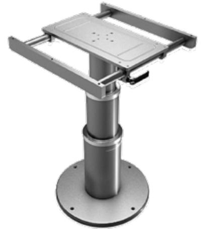
**Two-stage 6" Electric Pedestal with sliding upper plate to adjust table distance from seating.** Built in polished, brightened and anodized light alloy Sliding upper plate with 7.8" stroke to adjust the table distance from seating The generous size of the tubes and bases make it ideal for tables of large dimensions. The two stages telescope enables to get a reduced minimal height, often necessary to transform a table in bed. Push 220 lbs.
