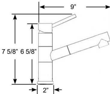
**Minimalistic Compact Mixer** for basin or small galley with swivel spout. Spout does **NOT** pull out. Ceramic valve. Spout tip rotates 360° left/right.
