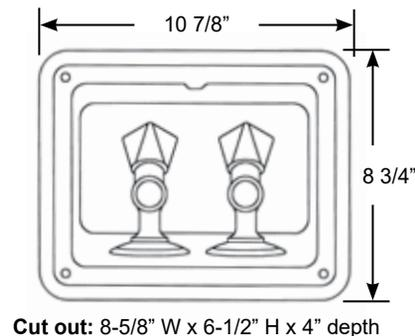
Flush mount boxes hide single and double wash down hose spigots. Minimal 1" protrusion beyond mounting surface. Thermo-formed, acrylic capped ABS box with incorporated hinge features one or two wash down spigots. Double spigot version makes a great fresh and salt water wash down station. Mounting hardware included.
