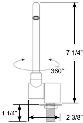
Fold-down Spout for foot pump. This faucet has no on/off valve.
