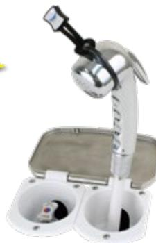
**#12144 Chrome Euro** spray handle with 6' white nylon hose, push trigger down for on/off or lock up for continuous water flow.
