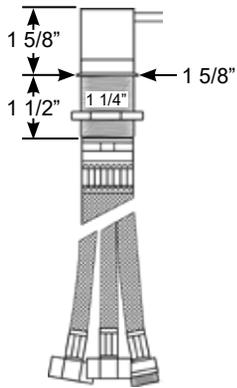
**Single Lever** on/off valve (Cold Only) , this valve is designed for use with our Push-Button or Euro trigger pull-out shower handles (see **#12139** and **#12145**). With the water pressure turned on simply rotate the valve to turn on the sprayer.
