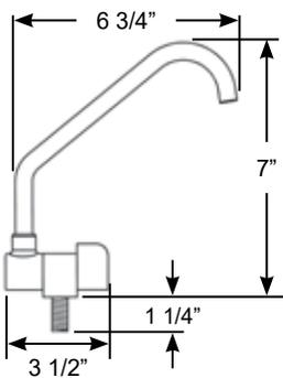
Folding **COLD WATER** Tap with Double Bend Swivel and Folding Spout. Ceramic valve.
