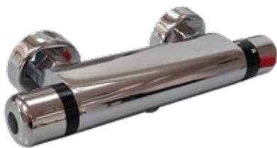
**NEW Thermostatic Mixer Heavy Type.** Features temperature control with a locking button at 100.4°F. Automatically maintains the water temperature output for the shower with incoming water supply temperature fluctuations. This fixture acts as an anti-scald device.
