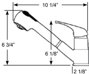
**Single Lever** swivel spout galley mixer with pull-out sprayer. Push-button spray pattern adjustment located on spray handle. 5' chrome-flex hose. Ceramic valve.
