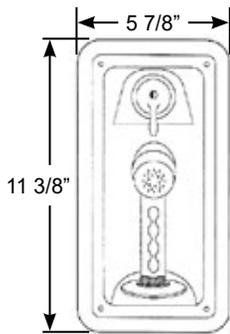
Vertical shower cavity (no door) with single lever mixing valve. One piece molded acrylic capped ABS. Off-white color #12 to match most off-white hulls. **Euro** sprayer handle attached to 13' nylon hose. Mounting hardware included.
