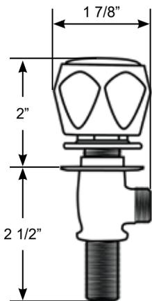
**Compact COLD WATER** tap for shower control. Bulkhead or counter top mount. (Max mounting surface thickness 1/2") 10015 1/2" adapter included.
