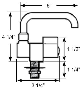
Folding **COLD WATER** Tap with low swivel and folding spout. 1/4 turn ceramic valve.
