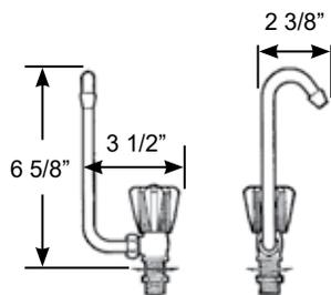
Folding **COLD WATER** Tap. Ideal for installing in a sink, under a seat or in a bait station. Vertical or horizontal installation.
