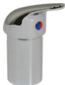
**Single Lever Shower Mixer** with an extended reach. Can be mounted on bulkhead or counter. 3/8" BSP-M flexible output supply line for hose connection.
