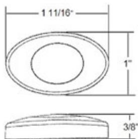
**Small Size Surface Mount 2-LED Light with Polished 304 Stainless Steel trim.** Suitable for interior or exterior installation. Stainless Steel mounting screws included.
