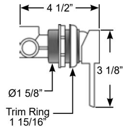
**Elka Mini-Compact** Bulkhead Mount Spout with Mixer and trim plate with BLUE LED accent on edge of trim plate. Ceramic valve.
