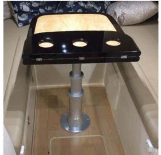
**Two-Stage 4" Telescopic, Through-the-deck, Electric Table Pedestal.** This version has a lower main tube which can be slid down through the base to obtain a lower minimum and maximum height. Total stroke is 15-3/4". Suitable for exterior applications. Maximum capacity is 220 lbs. Maximum table dimensions 2' x 3'.
