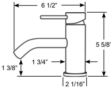
**Nordic Stainless Steel** Galley or Basin Mixer made of durable, low maintenance **Passivated 304 Stainless Steel**. This light weight faucet is perfect for installation on flybridge or aft cockpit locations. Ceramic valve.
