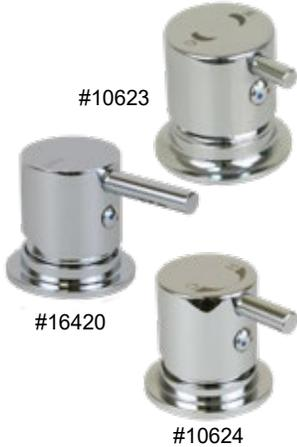
**Single Lever Mixing Valve WITH or WITHOUT** an on/off control. #16420 and #10624 operate by lifting the handle however, #10623 mixer is designed for use with the water pressure turned on simply rotate the valve to adjust the temperature.
