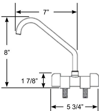
**Water Connection:** 3/8" BSP-M threaded shafts, 1/2" NPS-M adapters included
