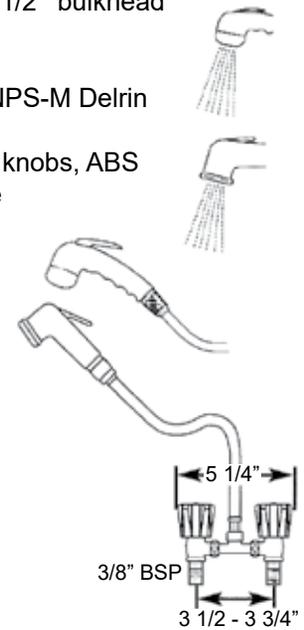
Complete shower kit. Includes mixing bridge, shower handle with on/off, 5' chrome-flex hose and bulkhead holder. Available with white or black shower handle. Mixer is shown as a bulkhead mount. Same unit can also be counter-top mounted.
