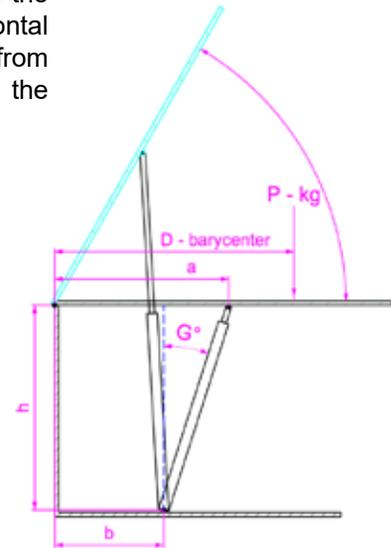
**It is evident that the thrust varies greatly according to the chosen assembly**, and that the most favorable conditions are obtained by applying the thrust point as far away as possible from the hinges and with the actuator in a position perpendicular to the closed hatch.
