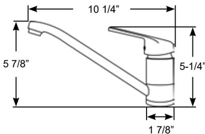
**Water Connection:** Flexible supply lines with 1/2" NPS-F fittings
