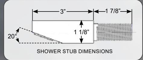
Scandvik's **NEW Shower Stub** is a simple solution for hardtop and bulkhead mount showers. Pair with Scandvik's shower mixers or a solenoid valve and switch. The scale resistant sprayer aerator can be removed for powder coating and service.
