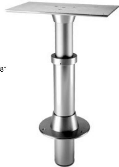
**Single-Stage, 4" Through-the-deck, Electric Table Pedestal**, has an adjustable, through the deck, periscope base which allows for lower minimum height. Table will swivel and lock with under-top handle. Maximum under deck area needed is 14.34" Maximum capacity is 220 lbs.
