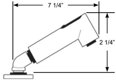
**Pull-out sprayer with Adjustable Water Flow.** A valve with a shut off is needed with this shower.
