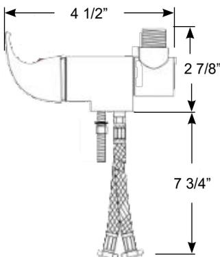
**Single Lever** mixing bridge. Features inward opening valve handle to prevent accidental opening in rough conditions while underway. Hose attachment swivels to any angle for greater flexibility.
