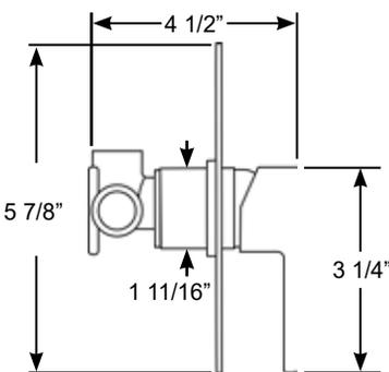
**Yo Bulkhead Mount Shower Mixer** with large square trim plate. Requires securing fixture inside bulkhead. Installation requires 2-3/4" behind front of bulkhead.
