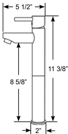
**Minimalistic** Raised Deck Mount Mixer for vessel sinks. Ceramic valve.
