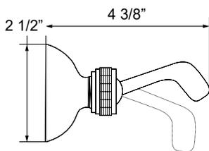
Adjustable bulkhead holder for **STRAIGHT** shower handles. Swivels 360 degrees for better adjustment.
