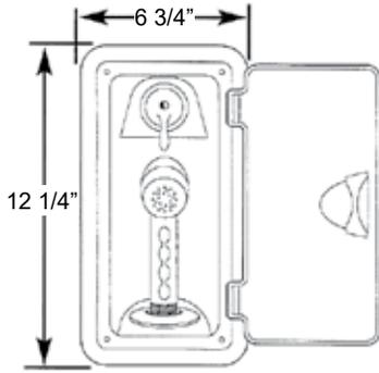
Vertical shower box with single lever mixing valve. **Euro** sprayer handle with nylon hose. Mounting hardware included.
