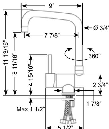
**NEW Nordic Family Folding Galley Mixer.** Folding spout is equipped with an aerator and swivels 360 degrees. Folds for cabinetry access!
