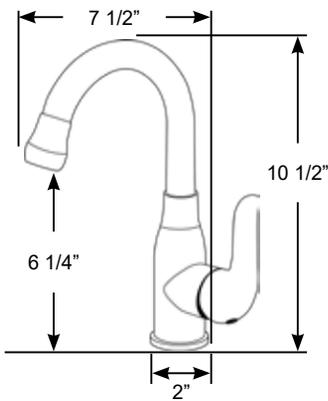
Made of durable, low maintenance Passivated 304 Stainless Steel. This light weight, compact faucet is perfect for installation for galley or bar. Features swivel spout.
