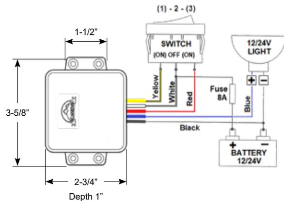
The **Tortuga Dimmer** is designed to easily adjust the interior or exterior light level from 0-100% output. Touch the “up” button to turn light on and touch the “down” button to turn light off.
