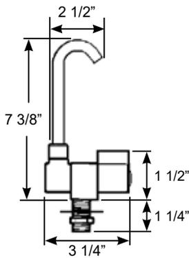
Folding **COLD WATER** Tap with High Reach Swivel and Folding Spout. Ceramic valve.
