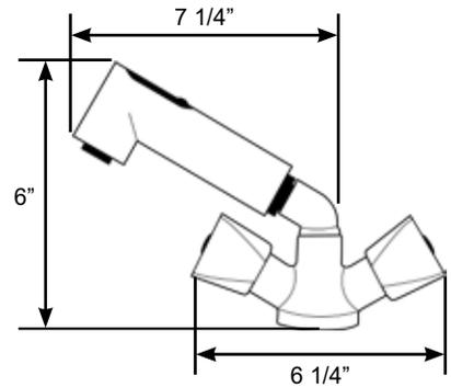
Combination faucet and shower with 5' pull-out hose. Press the button on back of handle to switch between aerated water flow or shower spray. 1/4 turn ceramic valves.
