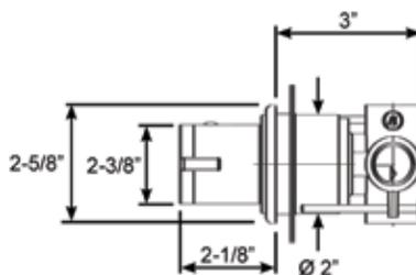
**Elka Diverter** for directing water from a mixer to either of two shower fixtures. Requires securing fixture inside bulkhead.
